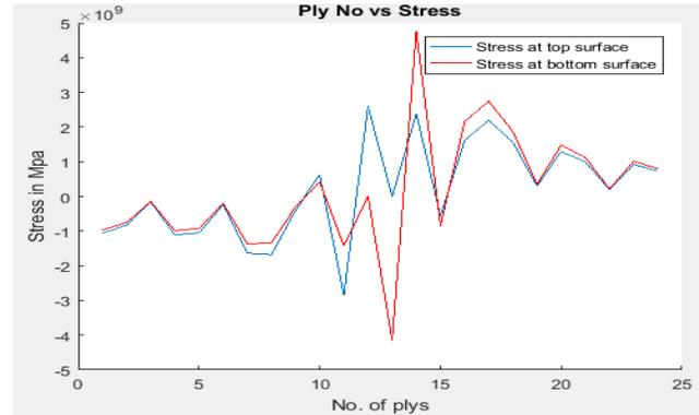
**Fig. 5: Stress variation with ply number for Cantilever beam**
