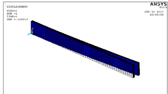
**Fig. 6 Deflection of Cantilever Beam**
