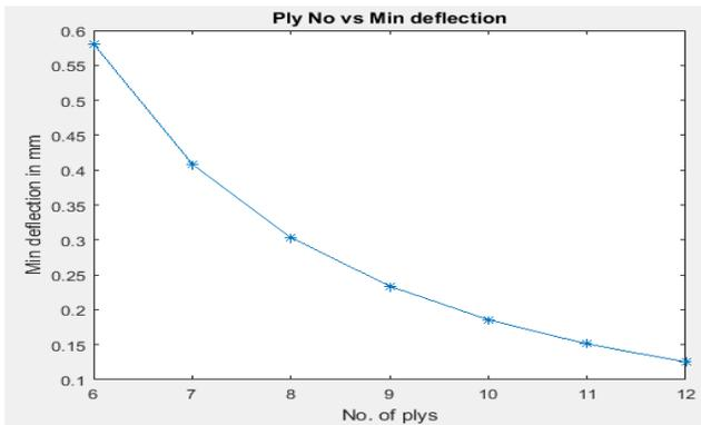
**Fig. 4: Minimum Deflection Vs Number of plies for Cantilever Beam**
