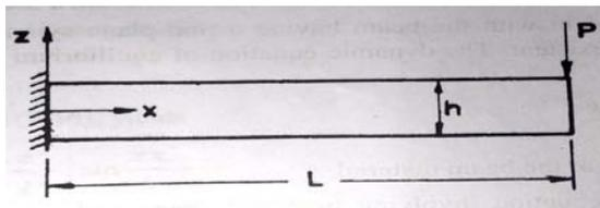
**Fig. 3: A Cantilever Beam for design Analysis**
