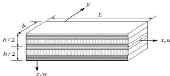
Fig. 1: Composite Beam laminates.
