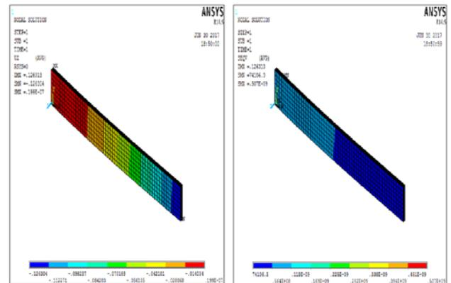
**Fig. 7: Z- Component of displacement and Von-misses stress of beam**
